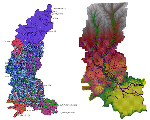
Figure G-1 – HEC-HMS Model Geometry (left) and HEC-RAS Model Geometry (right)
